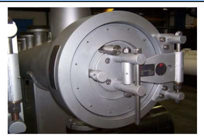
Closures are pressure retaining structures designed to provide access to pipelines and pressure vessels. Pipeline Engineering has developed the Rapid Opening Closure (ROC) to provide fast access to pipelines and pressure vessels. Designed and manufactured by our dedicated closures team, the Rapid Opening Closure is an ideal access mechanism to pipe line complexes.
