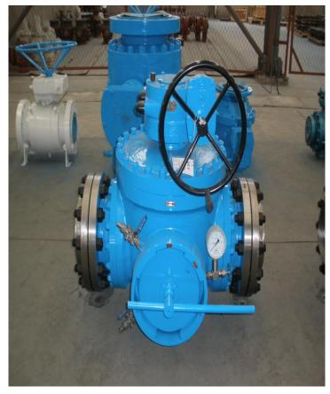
100% pressure testing on all of our Pig Valves. Designed in accordance with ASME B16.34, API, and NACE requirements.
